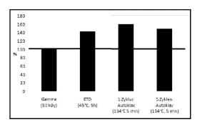
The diagram above shows the tensile shear strength of Al/Al bonding after sterilization expressed as % from the initial value. The specimens were cured by exposure to 80 °C for approximately 20 min.
